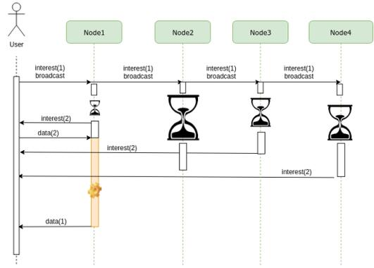
Fig. 2. The user asks the network to offload a task via broadcast. Node1, the fastest, replies with an interest asking for the code+input, Node2 spoofs Node1's packet and stops its flow, while Node3 and Node4 reply anyway. Node1 computes the program and sends the output to the user.
